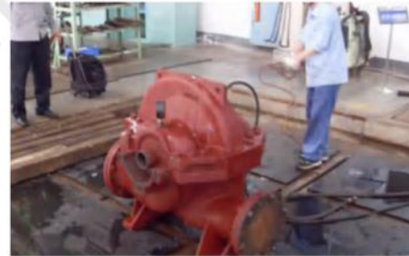
PN.4 Hydrostatic Testing
