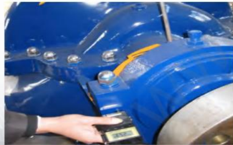
PN.7 Film Thickness Testing
