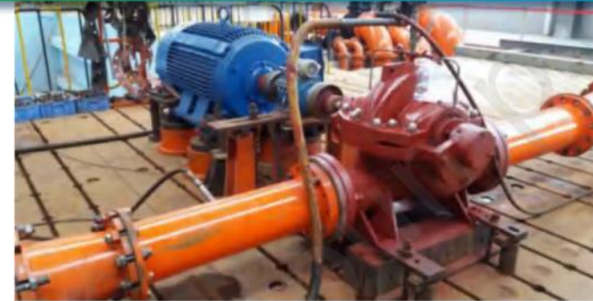
Double-suction Split Casing Pump Hydraulic Performance Testing
