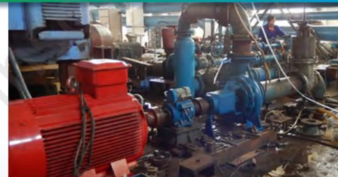
End-suction Pump Hydraulic Performance Testing
