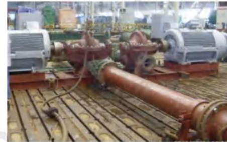
PN.5 Double Suction Split Case Centrifugal Pump Testing
