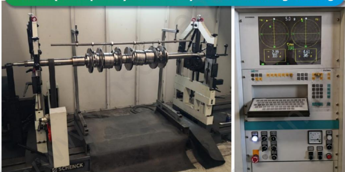
Rotor (or Impeller) Static & Dynamic Balancing Testing
