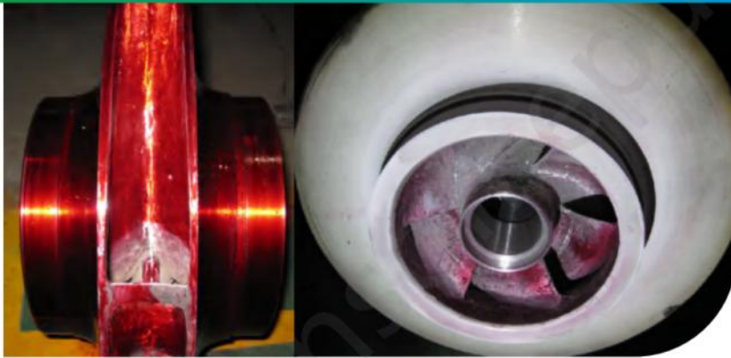
PT: Liquid Penetrant Inspection / Impeller
