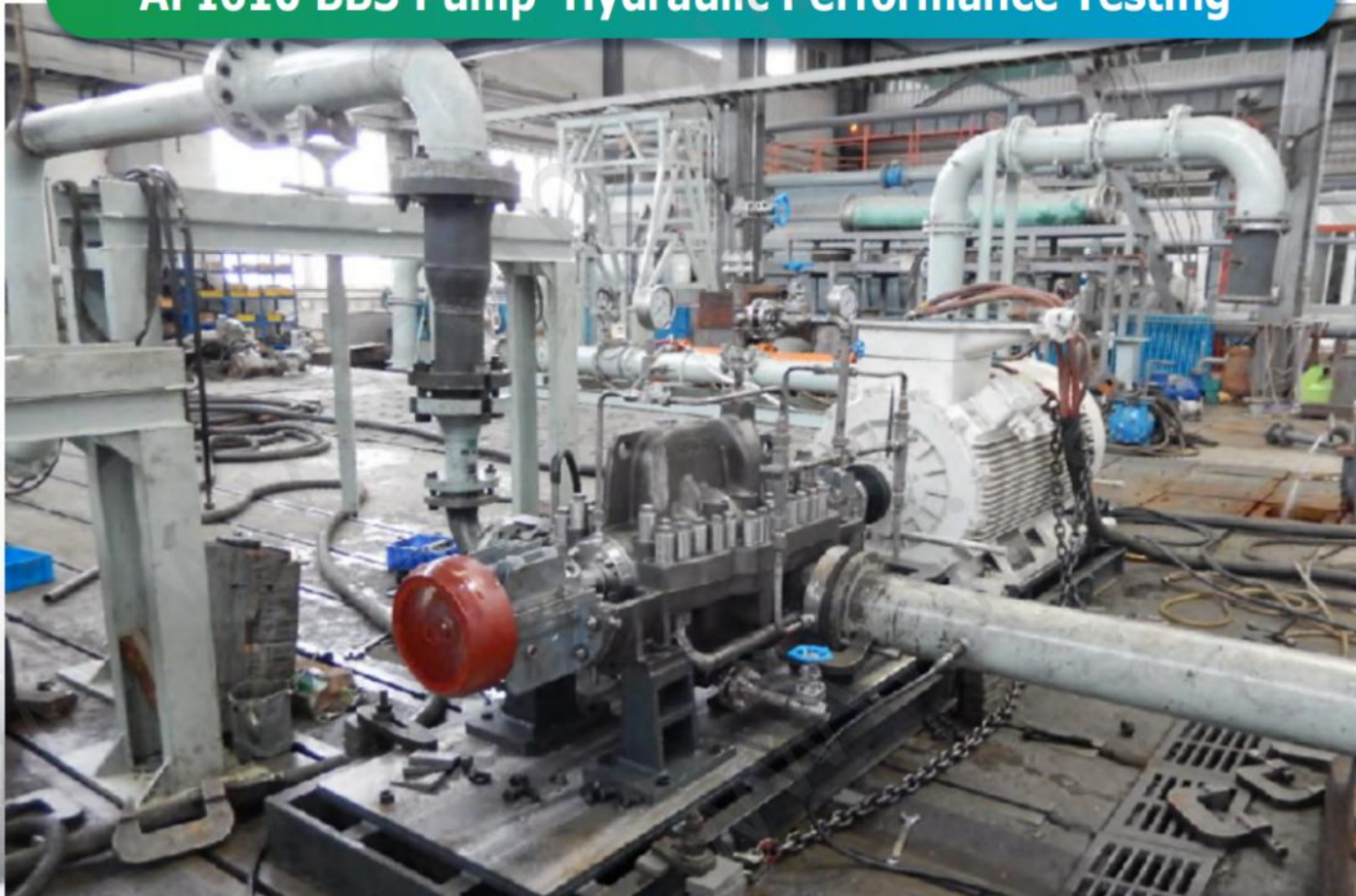
API610 BB3 Pump Hydraulic Performance Testing
