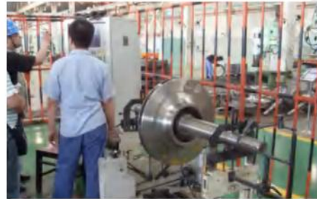
PN.3 Impeller Static & Dynamic Balance Testing
